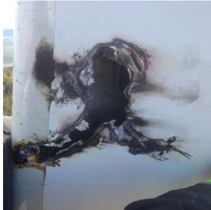
Figure 12: A consequence of having a thermal heating system at a blade [17].
