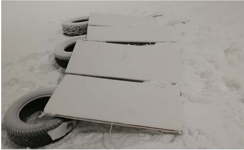
Figure 32: Snow build-up for small scale tests.
