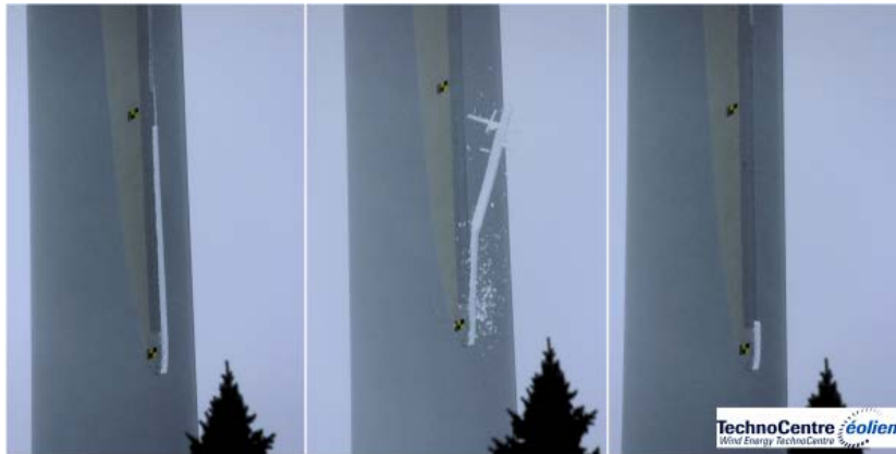
Figure 5: A sequence of ice falling from a wind turbine blade [11].
