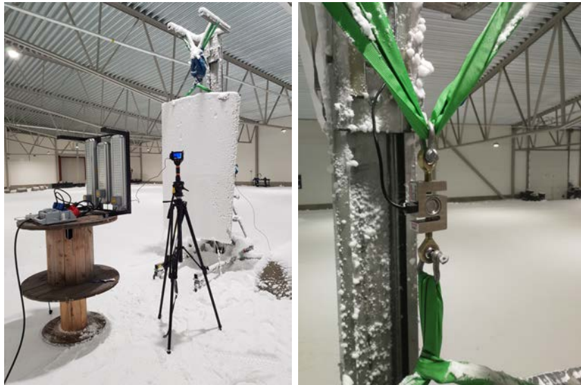
(a) Hanging blade, heaters and (b) Close up of the load cell and suspension device.
