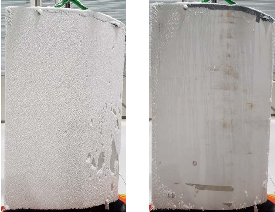
(a) Surface of blade before de-icing. (b) Surface after de-iced blade.
