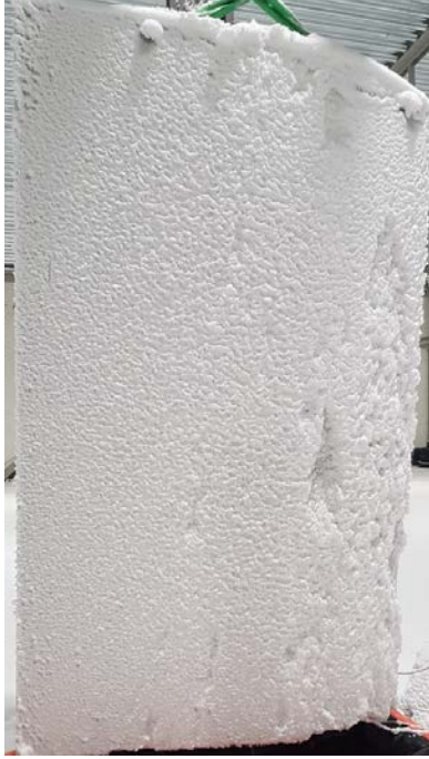
(a) Surface of blade before de-icing. (b) Surface after de-iced blade.
