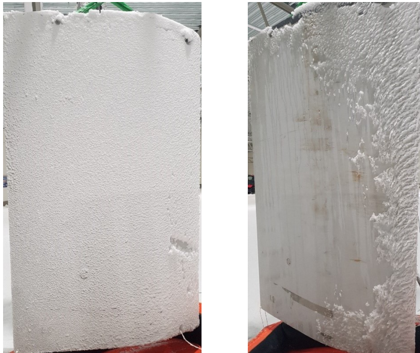
(a) Surface of blade before de-icing. (b) Surface after de-iced blade.
