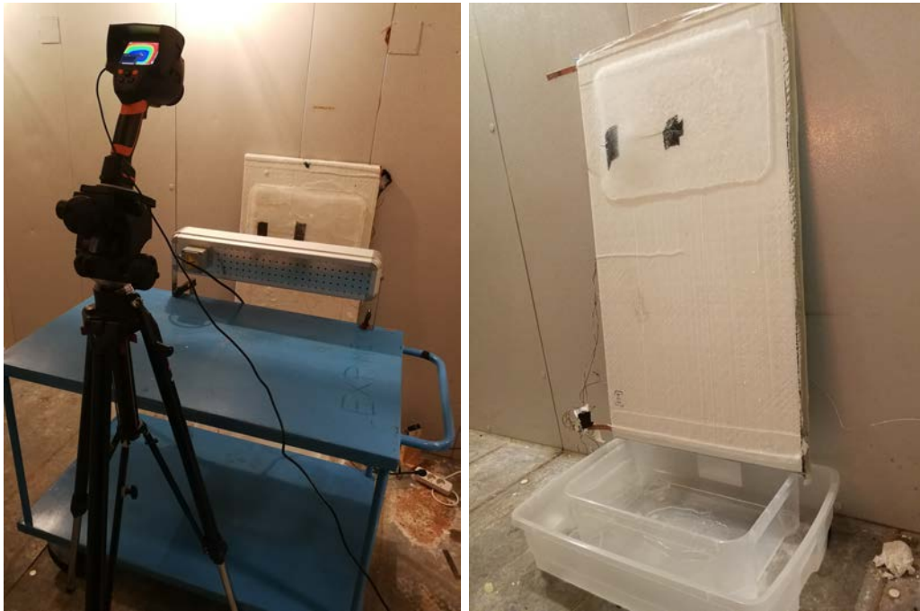
(a) The setup with camera, heater and blade. (b) The blade with plastic boxes to collect melt water.
