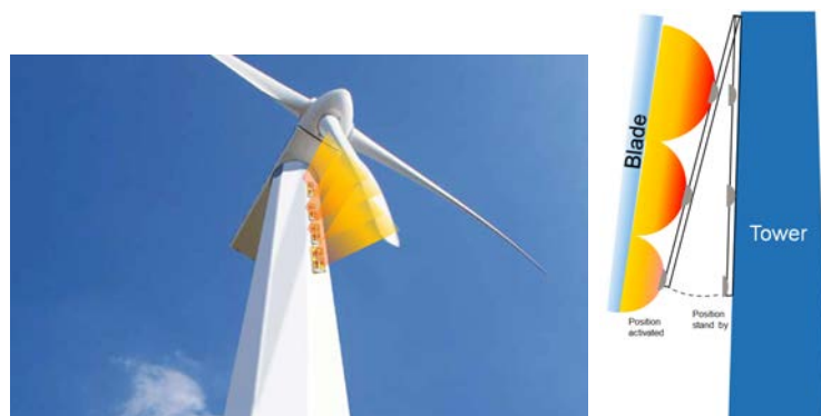
(a) Placing on the tower.
