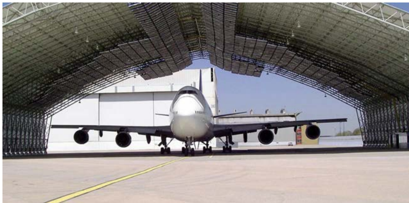
Figure 14: De-icing of airplane with IR-heaters at JFK International Airport [24].
