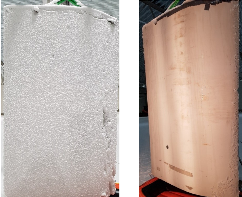
(a) Surface of blade before de-icing. (b) Surface after de-iced blade.
