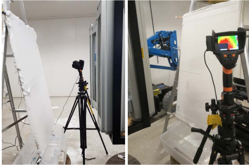
Figure 33: Experimental setup for the small scale test with snow.
