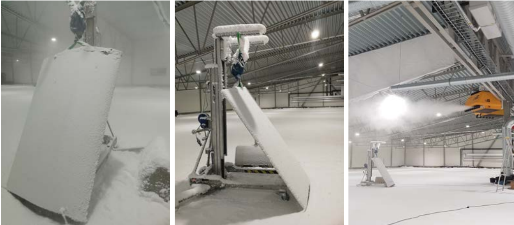
Figure 34: Snow build-up for the full scale tests.
